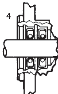
DOUBLE SEAL WITH OVERBOARD DRAIN
